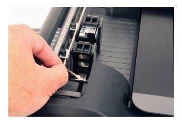
4. Slide the cartridge into the cartridge holder "feet first" then press the top of the cartridge firmly into the cartridge holder until you feel two clicks. This ensures that the cartridge is fully seated.
