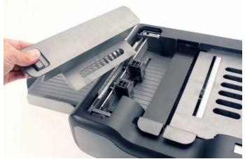
2. Notice the location of the cartridge holder that is inside the printer assembly. Also notice the ruler, the printer alignment mark, and the thumbscrew that sit beside the cartridge holder. These are the elements used to position the printer(s).
