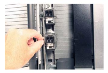
**5.** Move the printer to the 1.6 inch position and lightly tighten the thumbscrew.
