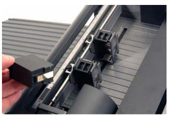
3. Using a clean swab, gently wipe the area of the cartridge holder that contains the electrical contacts.
