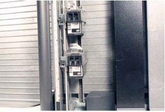
4. Loosen the thumbscrew so that you can move the printer.
