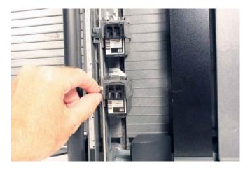
5. Move the printer to the 1.6 inch mark and lightly tighten the thumbscrew.
