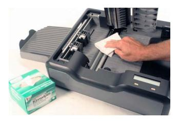
**NOTE:** Single read head units do not have glass beneath the top read head. Instead, they have black, shiny strip. This must also be cleaned.
