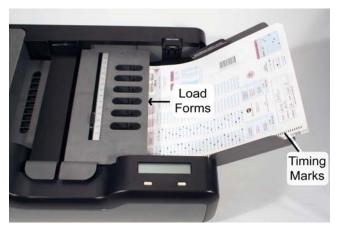
7. Follow the instructions in the *Scanning Tests, Ballots, and Surveys Using SelfScore* guide to scan the type sheets that you just loaded.
