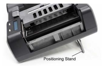
2. Ensure that the input tray and output tray (or Select Stacker) are in place and that the adjustment bar is properly positioned for the sheets being scanned.
