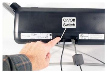
2. After you turn on the scanner, wait for it to complete the self-test. The message "Initializing..." will appear on the display panel. After a few seconds, another message will appear indicating what action needs to be taken next.
