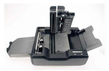
2. Spray canned air (with a non-condensing propellant) directly on the transport bed area. This removes large amounts of dust and other types of debris.
