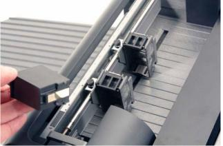
Slide the cartridge into the cartridge holder "feet first" then press the top of the cartridge firmly into the cartridge holder until you feel two clicks. This ensures that the cartridge is fully seated.
