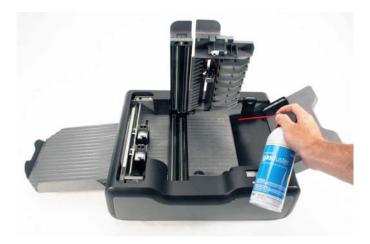
3. Clean out any dust or debris that has collected in the area between the top and bottom read heads where it is hinged using canned air.
